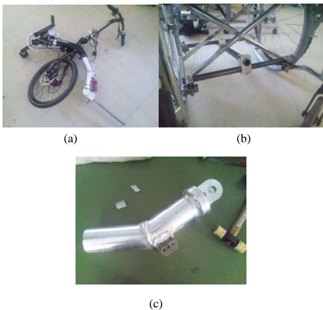
Fig. 3 Improved front unit (a) adapter unit (b) welding part of front unit (c)
