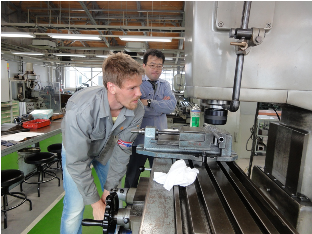
Figure 14. Drilling inner pipe adjusting holes
