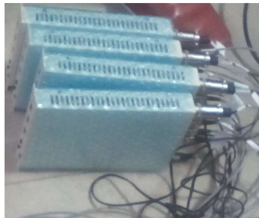
Amplifier that was directly connected to the 6 axis-sensor
