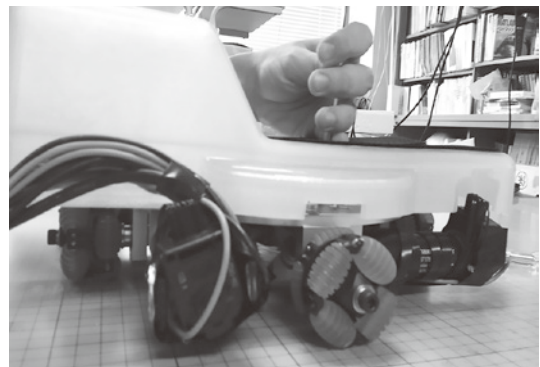
Fig. 3. Omni wheel to move the robot in all directions
