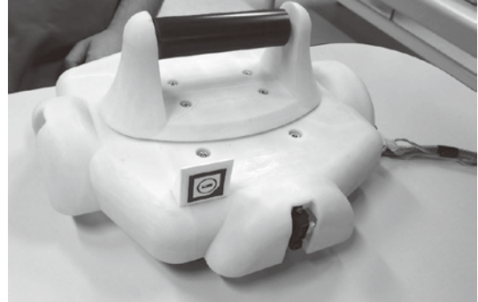
Fig. 2. Rehabilitation robot and AR marker placed on it
